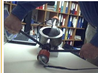
Tube Extruder Die shown with dual driving transducers
