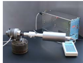
Plastic Extruder Head, Ultrasonic Transducer and MMM Generator
