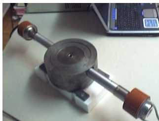
Tubes Drawing Die and Ultrasonic Transducers
