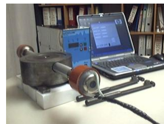
Tubes Drawing Die, MMM Generator and Transducers
