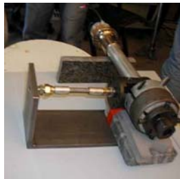
Plastic Extruder Head & Ultrasonic Transducer
