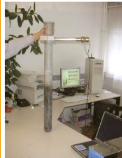
Clamp-On Ceramic tube for Liquid Metals Treatment
